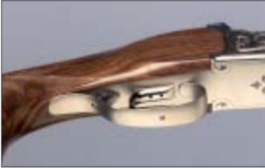
To adjust the trigger position, loosen the screw about one turn with the hex key provided (See image). The forward opening in the trigger is where the screw is. The rear opening does not contain anything. Slide the key to the desired position and gently retighten the trigger position screw.
