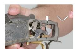
The safety of the K-80 and K-20 can be locked in the "off safe" position and made inoperative. The purpose of this feature is to prevent the loss of a target in competition that results from inadvertently leaving the safety on. This feature is for use ONIY under the controlled conditions
