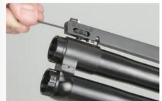
HOW TO LOWER AND RAISE THE RIB Loosen the locking screw at the very front of the rib which locks the adjustment wheel (see illus. page 14). Use the 1.5 mm allen key supplied and remove the locking screw completely. The adjustment wheel is now free to turn. To raise the POI, turn the wheel clockwise in order to move the rib down.
